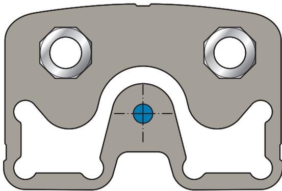
Flexible plate bars allow durable deforming for precise adjustments in final production phase.
