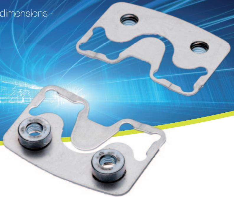
Nedschroef's anchor plate combines a robust and durable fixation area with the possibility for tolerance adjustment - in one single part. This is done by deforming the flexible bars in the plate. Our unique solution is applied in the automotive industry for the adjustment of door locks, at the end of the assembly process, allowing the customer to make precise adjustments in the final phase of production.
